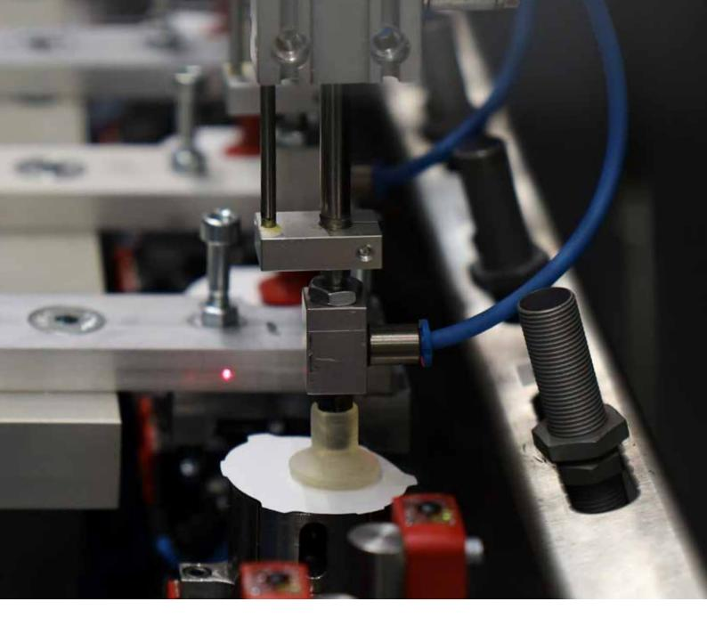
A liner could be everything from a simple foam disc to a combination of several different materials. There are liners which are welded to give extra protection from moisture and oxygen, and at the same time ensures the final user the product has not been opened.
